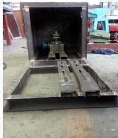
**Gambar 6.** Rangka Mesin *Pellet Maker Four Roller System*
