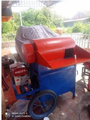
Gambar 12. Proses Assembly Mesin Perontok Padi Sistem Lorong Hembus
